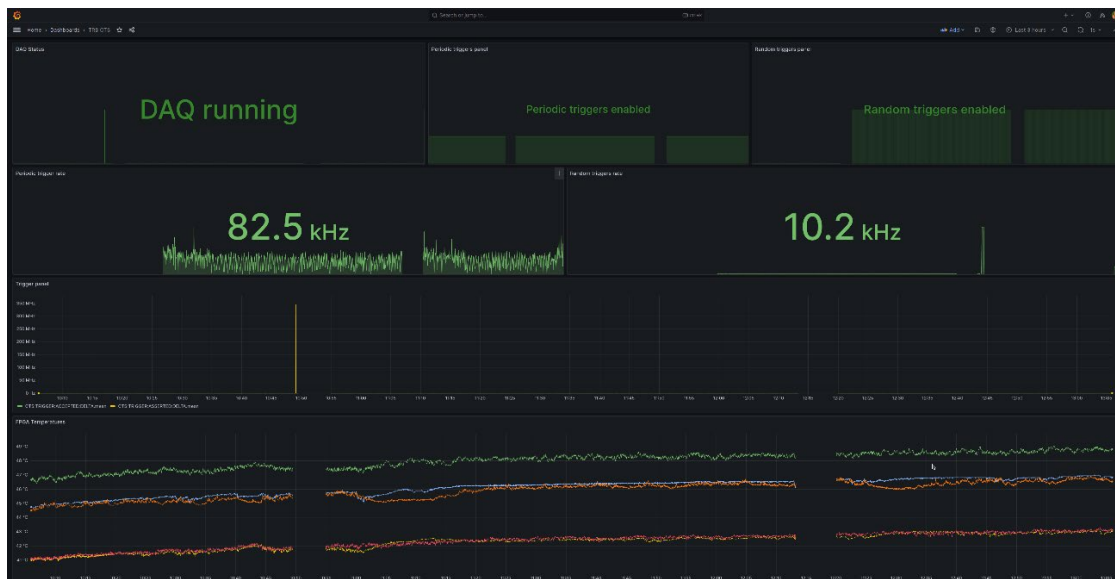
Figure 2: Grafana TRB3 Central Trigger System monitoring dashboard
