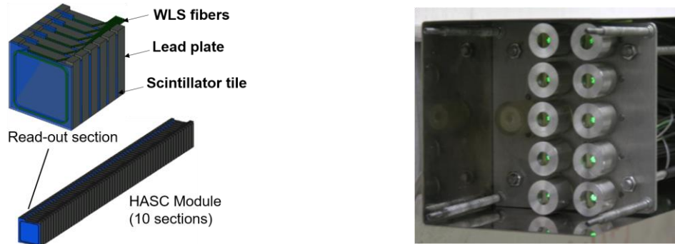
Figure 3: HASC module longitudinal section (left) and optical readout couplings (right)
